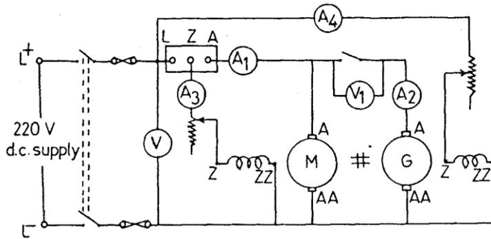
*Fig ‘A’ : Schematic diagram for Hopkinson’s test on DC machine.*
