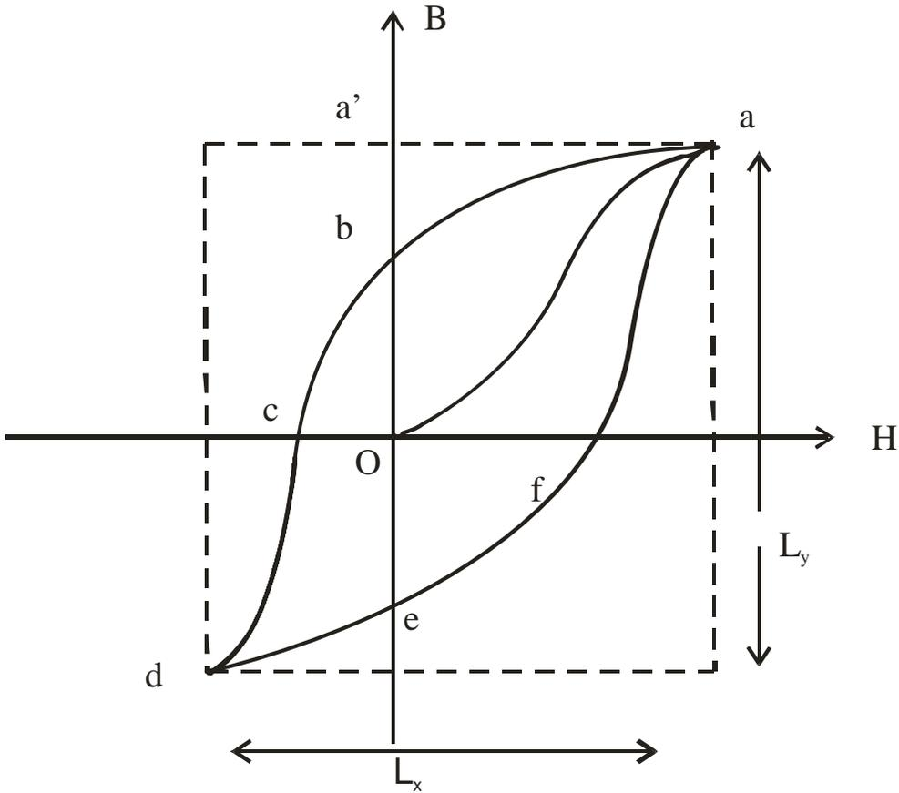
Fig.(2) B-H Curve tracing taken on tracing paper
