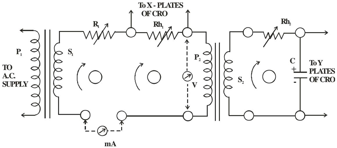
Fig (1) Circuit Diagram for obtaining B-H curve on CRO screen
