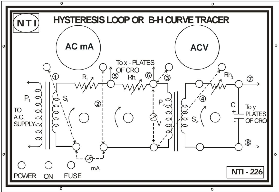
**Fig.(4) Connections for Hysteresis Loop or B-H Curve Tracer**
