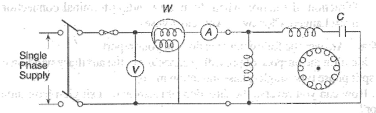
*Fig-‘3’ : Connection diagram for determine the effect of capacitor on the performance of a single phase induction motor.*
