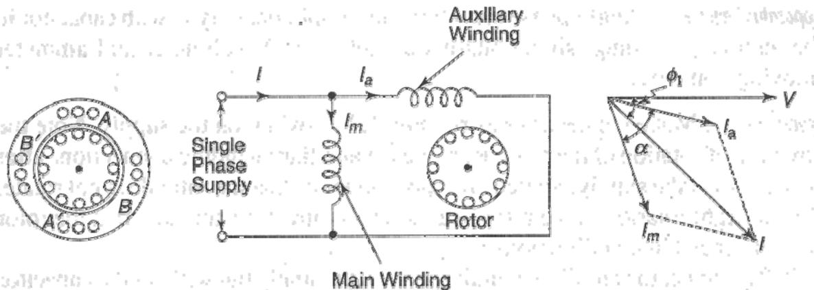
**Fig- '1' : Single Phase Induction Motor winding carrying currents which have a time phase difference of  $\alpha$  degree.**
